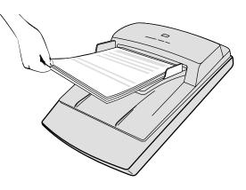
2 Adjust the paper guides to center the stack.
